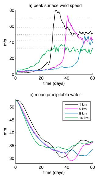
FIG. 8. Example time series of (a) maximum surface wind speed and (b) domain-mean precipitable water at different horizontal resolutions in rotating domains. All are for runs conducted on an fplane at 20°N with a domain width of 1200 km. Horizontal dotted lines in (a) mark lower bounds of the five Saffir–Simpson intensity categories.
