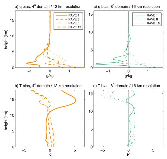
FIG. 4. As in Fig. 3, but showing how biases change as the RAVE factor is increased. (a),(b) Bias in 12-km-resolution integrations relative to a 2-km-resolution integration without RAVE (i.e.,  $\gamma = 1$ ), all in 4°-wide domains. (c),(d) Bias in 16-km-resolution integrations relative to a 2-km-resolution integration without RAVE, all in 8°-wide domains. Legends in (a) and (c) show the values of  $\gamma$ .
