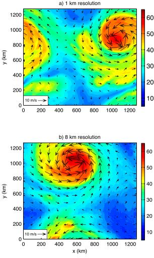
FIG. 9. Precipitable water (mm; color shading) and surface winds (vectors) in rotating domains for different horizontal resolutions, all without RAVE ( $\gamma = 1$ ) on the day when the tropical cyclone first achieves Saffir–Simpson category 1 at (a) 1- and (b) 8-km resolution.
