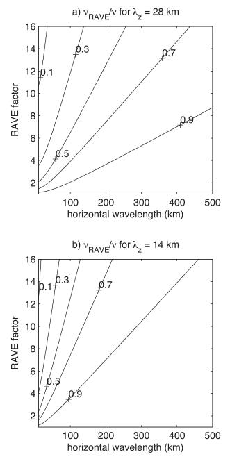
FIG. 6. Coefficient by which RAVE reduces the frequency (and thus the amplitude) of gravity waves with vertical wavelengths of (a) 28 and (b) 14 km.
