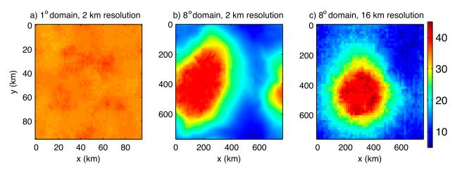
FIG. 1. Precipitable water (mm) in nonrotating domains 50 days after model initialization for different domain sizes and horizontal resolutions, all without RAVE (i.e.,  $\gamma = 1$ ). (a) The 96-km-wide domain at 2-km resolution, (b) the 768-km-wide domain at 2-km resolution, and (c) the 768-km-wide domain at 16-km resolution. Note the change in horizontal scale from (a) to (b) and (c).
