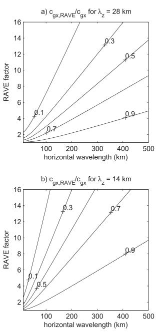
FIG. 5. Coefficient by which RAVE reduces the horizontal group velocity of gravity waves with vertical wavelengths of (a) 28 and (b) 14 km.
