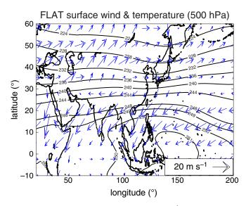
**Figure 3.** The simulated climatological surface wind (m s<sup>-1</sup>, arrows) and 500 hPa temperature field (K, contours) during boreal winter for the FLAT integration (with the large-scale orography removed and the gravity wave drag parametrization turned off). [Colour figure can be viewed at wileyonlinelibrary.com].
